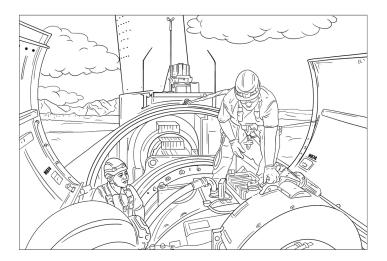
"That big blue thing you are leaning on is a gearbox and the thing you hit your head against on the way is the hydraulic union, which feeds oil into the pitch system through the gearbox into the hub from the hydraulic power pack down-wind. Behind that is a good place to poo and also the emergency exit. Next to that is the generator which is full of electrons but what we are interested in today is the caged beast behind you. That's the up-wind main bearing."
